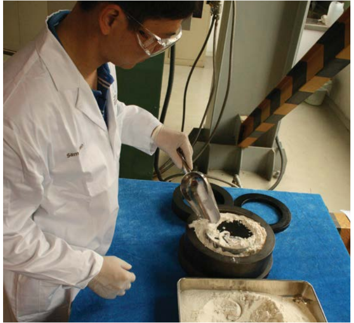
Clean tools must be carefully filled with the correct amount of VICTREX PAEK powder.
